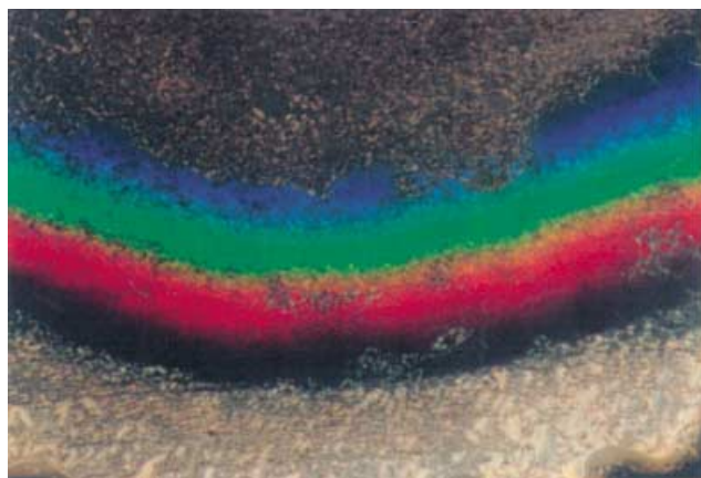
Figure 4. Selective reflection in a contact preparation between compound 4a and the nematic mixture MLC 6260. The color of the selective reflection changes according to Bragg's law because of a gradient of the concentration, which in turn leads to a variation of the helical pitch.
